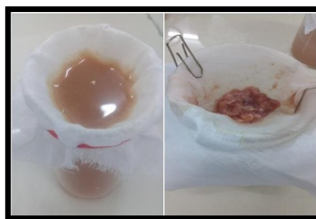
Figure 6: Muslin cloth to remove biomass
