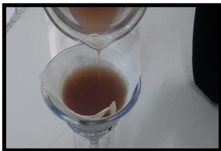
Figure 7: Filtration by using Whatman's filter paper number 1
